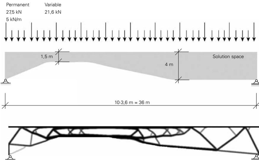
5. Generation of evolutionary optimised structural layout in constrained design space and the layout of the final (traditional) truss design for the renovation design of TU Delft faculty of Civil Engineering.
