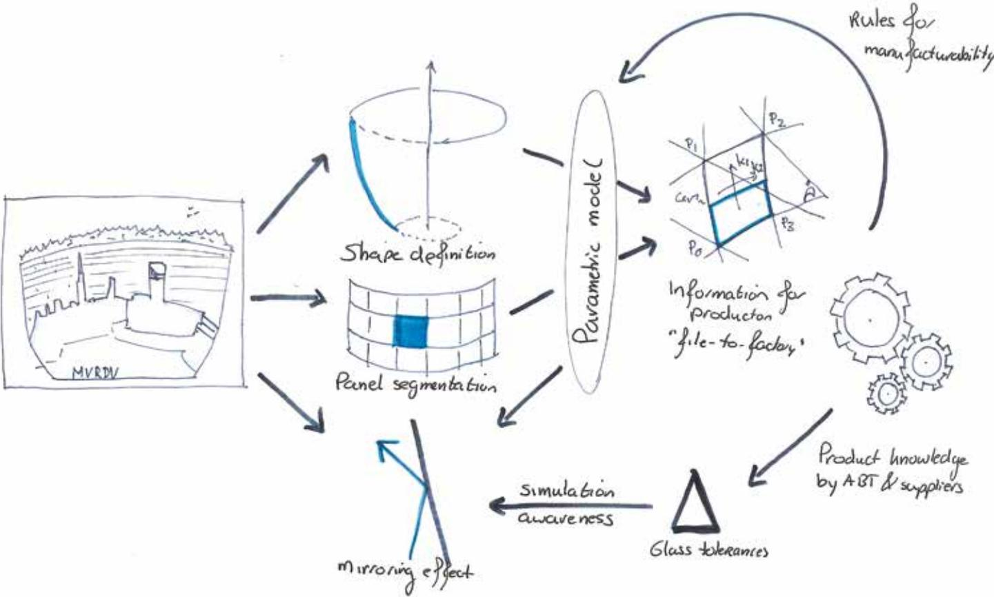
3. The role of parametric design in definition and control of geometry in the design process of Boijmans Van Beuningen Museum.
