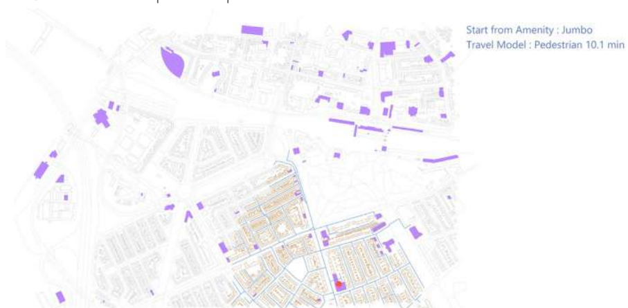
Figure 3: Mobility module: calculation of the street network within 15 min walk from a specific amenity.
